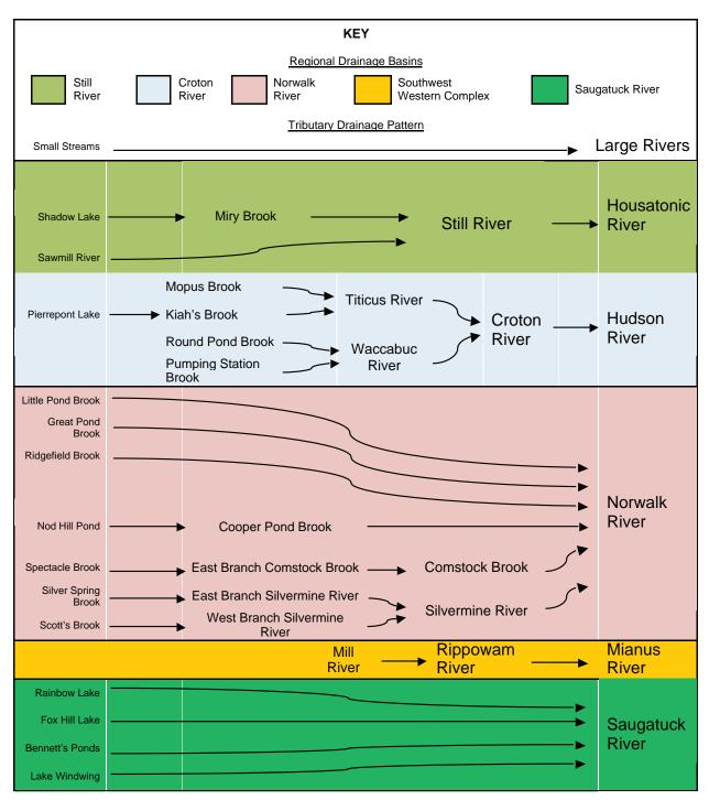
*Figure 3: Stream and river drainage patterns, Ridgefield, CT. The regional drainage basins are indicated by the colors noted. Flow path is indicated by arrows, with font size increasing with stream order.*
