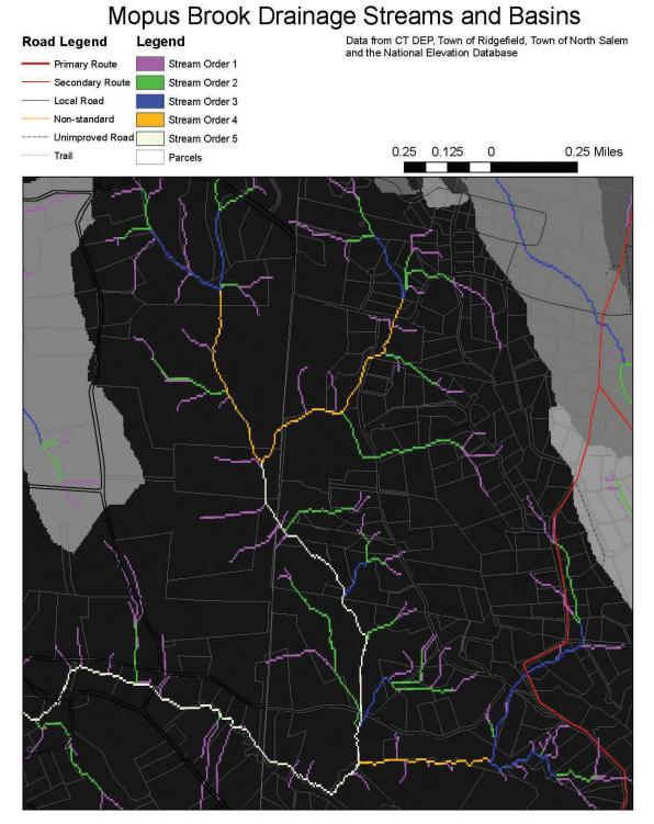
Figure 4: Stream drainage network, Mopus Brook. The shades in the background illustrate different drainage basins; only water from areas that are dark gray flows into Mopus Brook. The colors used for the brook and its tributaries represent stream order. Higher stream order indicates more tributaries. This map was created as a model, based on a digital elevation model (DEM) obtained from the National Elevation Database (prep. K. Amick).
